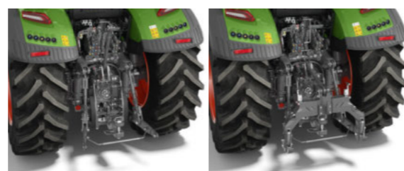
Rear linkage with ball ends and rub blocks
