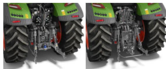
Rear linkage with quick catch hook and side support (EU)
